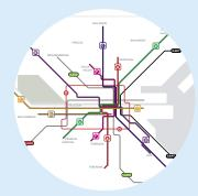
Redesign of the Dublin area bus network to provide a more efficient network with high frequency spines, new orbital routes and increased bus services.
