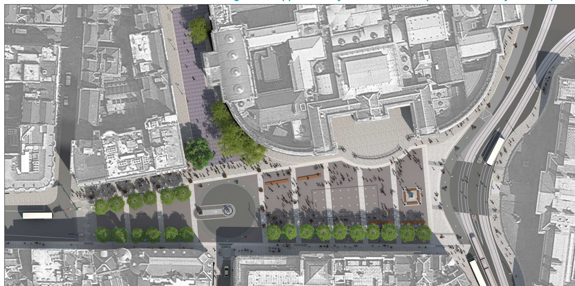
Figure 27: Proposed design for the College Green Civic Plaza. The path across College Green linking O'Connell Bridge and Dame Street will be closed to all vehicles, including buses. Approximately 120 to 150 buses per hour currently use this path.
