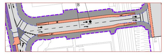
It is unclear how the proposed cycle lanes on Memorial Road interface with the cycle lanes on the adjacent road network, and in particular, how cyclists travel to/from the cycle facilities on the adjacent roads and those on Memorial Road.
