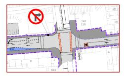
Eastbound buses on Emmet Road are likely to wish to proceed straight ahead at the South Circular Road junction, onto Old Kilmainham Road. To do this they must change lane from the bus lane into the straight-ahead lane on the immediate approach to the junction, a manoeuvre that is likely to be compromised should extensive queues form within the left-turning lane on this approach.
